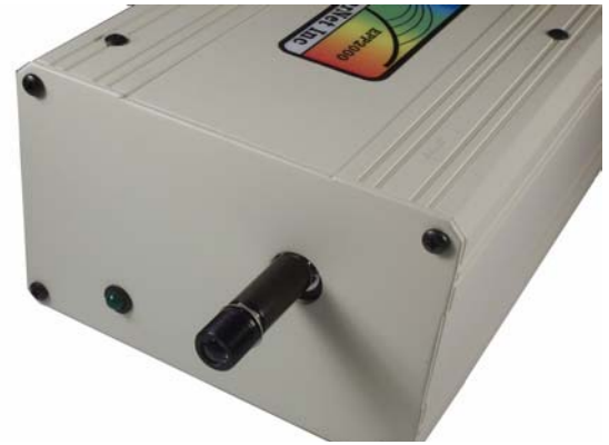
SMA-Coupler and Lens-QCol Directly on a Spectrometer
