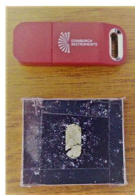
Figure 2: The diffuse reflection powder sample holder filled with Benzil powder (USB drive shown for size comparison).
