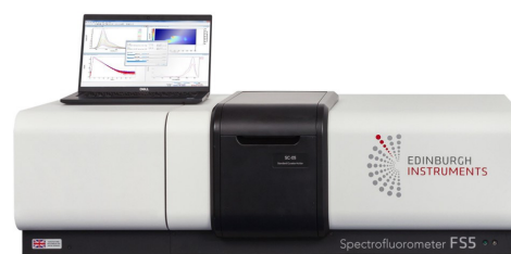
Figure 2 Edinburgh Instruments FS5 Spectrofluorometer.
